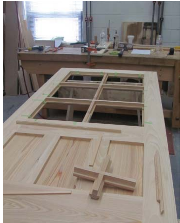
Replacement door using same materials, design and detailing as the original.
